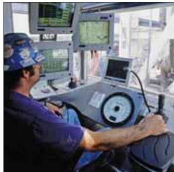
The driller's control cabin pictured here is part of an automated rig built specifically for EnCana.
