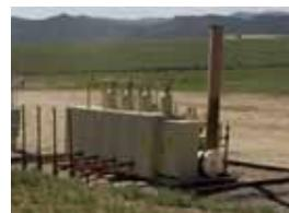
The Separation Unit removes liquid hydrocarbons and water from the gas stream. Natural gas located underground is very different from the gas used to heat homes and businesses. Natural gas that reaches the consumer is composed almost entirely of
